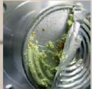
Process medium gets behind the diaphragm
