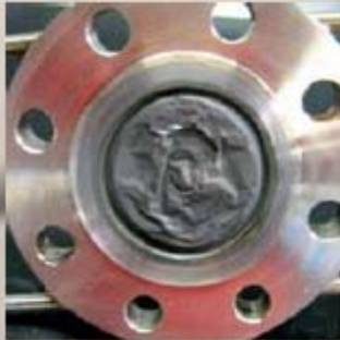
Diaphragm is "blown up"
